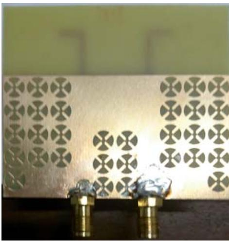
Figure 15. Fabricated (a) top and (b) bottom portions of the proposed low-RCS MIMO antenna.
