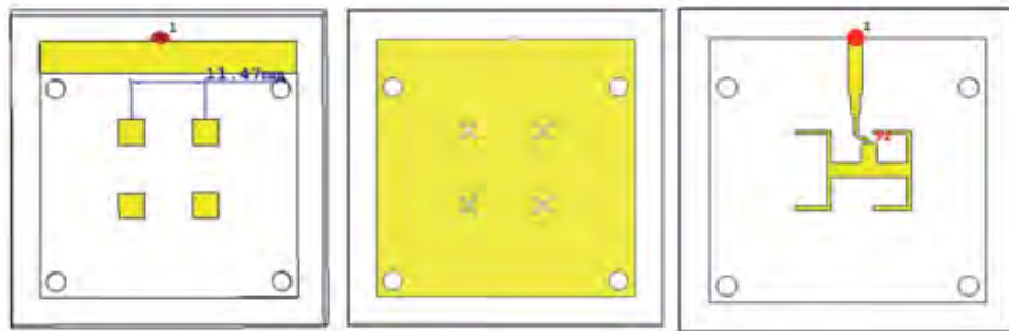
Figure 17. The antenna array implemented in CST MSW (front, ground, and back views).
