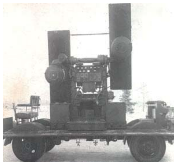
Figure 9. The radio-searcher B-3: the device for determining the elevation angle.
