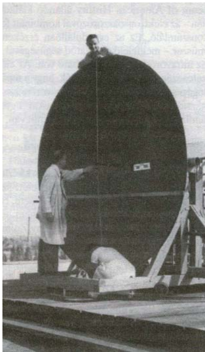
Figure 31. Antenna adjustment of the Borbála fire-control radar. Dr. Károly Simonyi is shown in front of the antenna [23].
