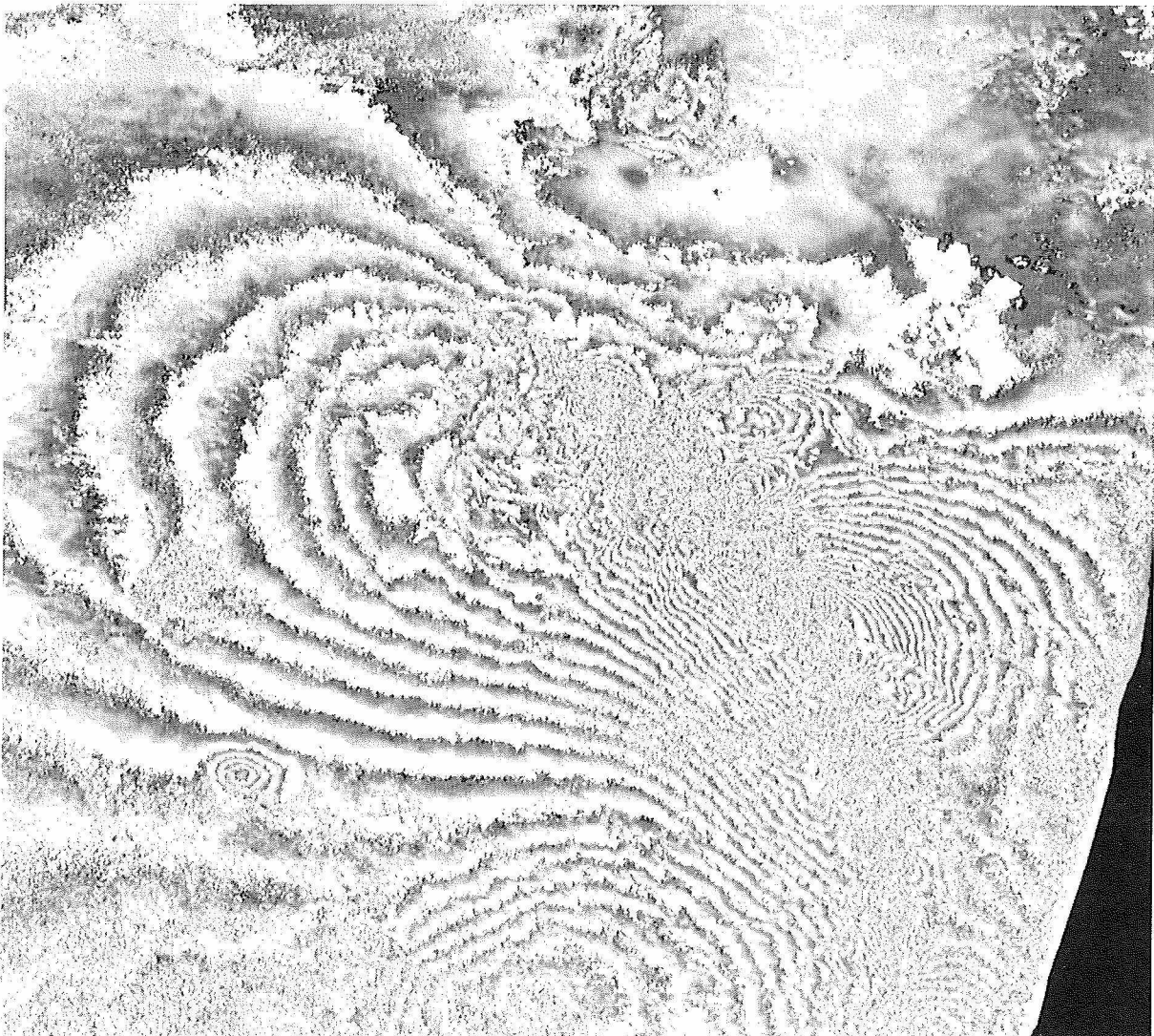
Fig. 2 - Example of topography revealed by SAR interferometry. The image shows the interferogram obtained on Awaji island [7], in Japan, using two radar images of the Japanese J-ERS radar satellite. The images have been acquired on May 31 and July 14, 1993 and were part
