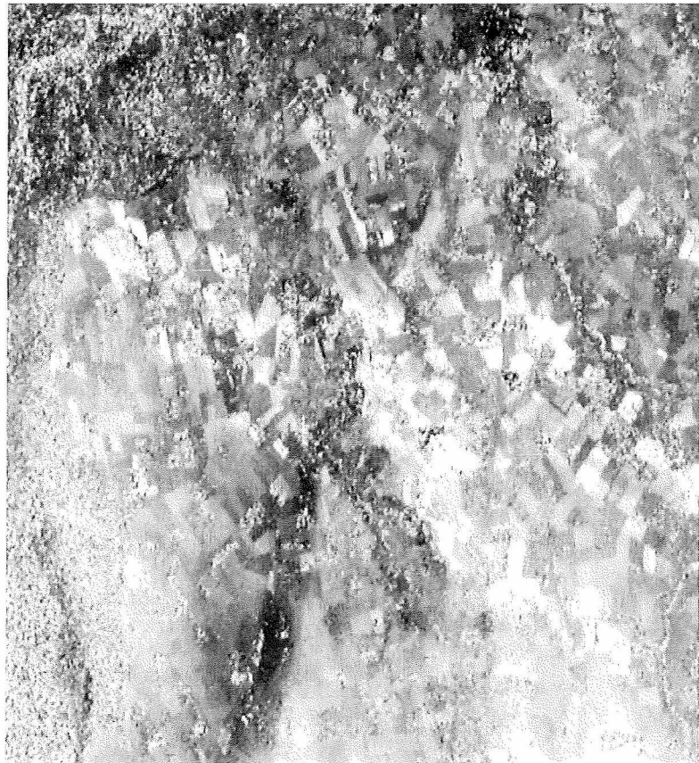
Fig. 8 - Surface phase changes associated with moisture on agricultural fields. This image was obtained from ERS-1 data, but the effect has been first observed with L-band Seasat data [4]. In the Seasat data case, the moisture was caused by irrigation. Here, it is likely to have been caused by rain. A brightness difference can be observed in the amplitudes of the images which form the interferogram over the area where surface phase change is sizeable. It is not clear whether the change is geometric (due to soil swelling under the action of moisture) or radio-electrical (due to moisture induced conductivity change).
